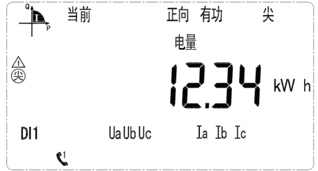
Current forward active energy 12.34kWh
