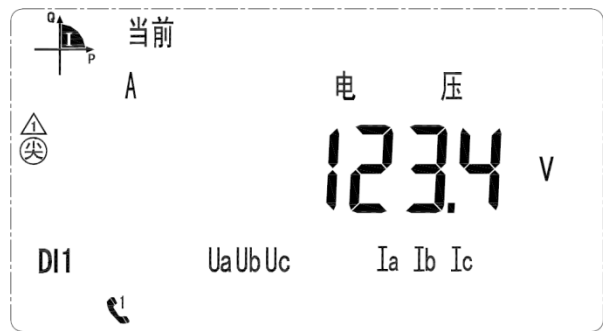
Voltage on A phase is 123.4V
